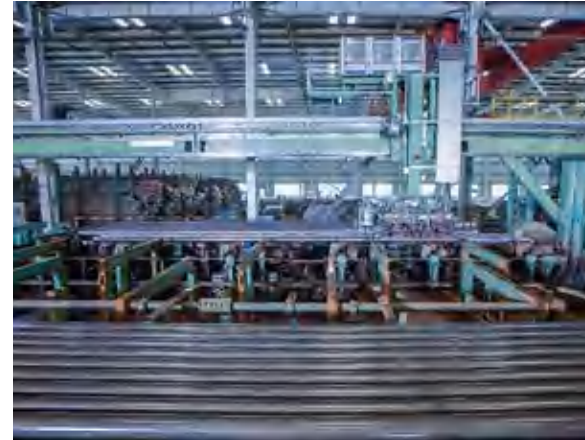
Drill Pipe Body Full Length Automatic Ultrasonic Test (FLUT)
